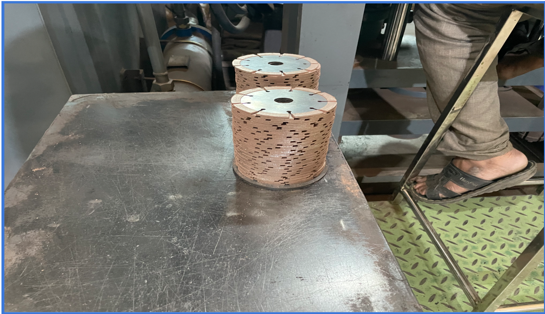
Fig.7 The baked blades after being put through the sintering process.
